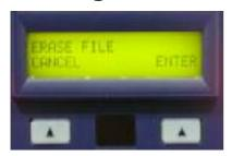
With this choice, the Soft Keys take on the options of **DELETE** and **CANCEL**. The file to be deleted is the current file indicated in the LCD display. Once the Soft Key under the word DELETE is pressed, the file is PERMANENTLY erased and the time code is reset to 00:00:00:00.
